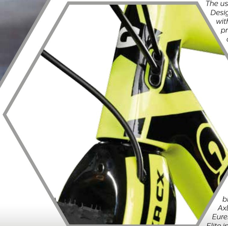
The use of these materials and innovative rear design (Cross Design Concept) guarantee greater frameset's elasticity, without reducing significantly torsional rigidity. This design provides a more reactive frameset in all the situations of relaunching the action, where in the cyclocross are frequent.
